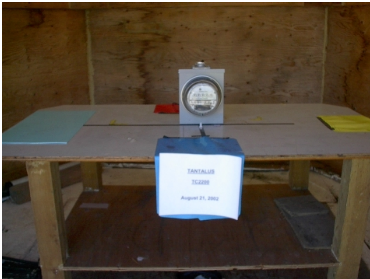
Emissions Test Setup Front View
