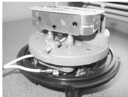
Figure 5: Connecting the module power leads to the meter power bus bars
