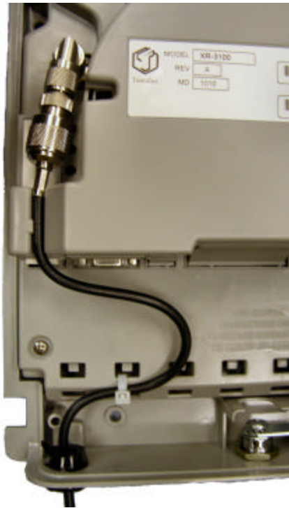
Figure 5 The XR-3100 with the strain relief correctly installed
