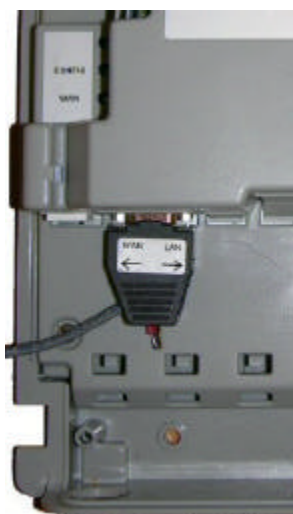
Figure 3 Switch position to select the LAN Controller.
