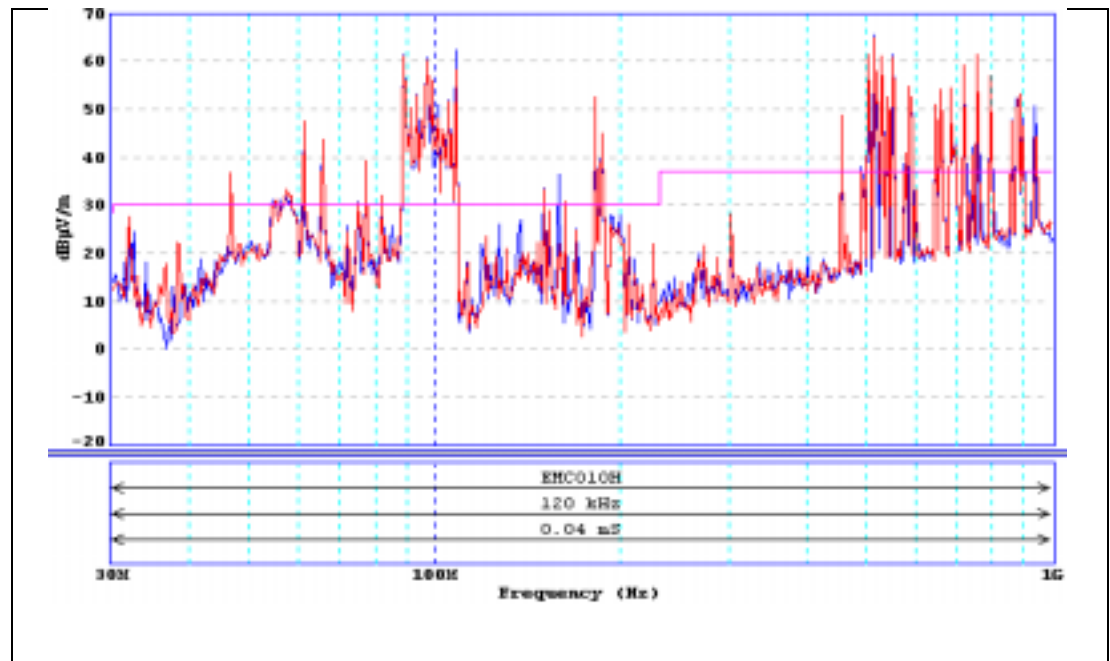
Fig. 8. The emission from the EUT's with a horizontally polarized broadband antenna 10-m from it. The antenna is 3.0-m up. Red is the ambient. The class B limit line is shown.
