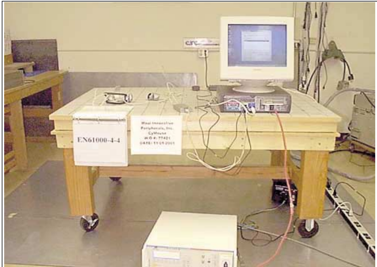
Electrical Fast Transient Burst - Power Lines
