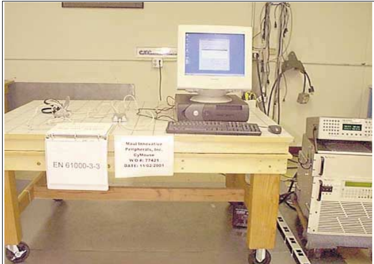
Voltage Fluctuations and Flicker Emissions
