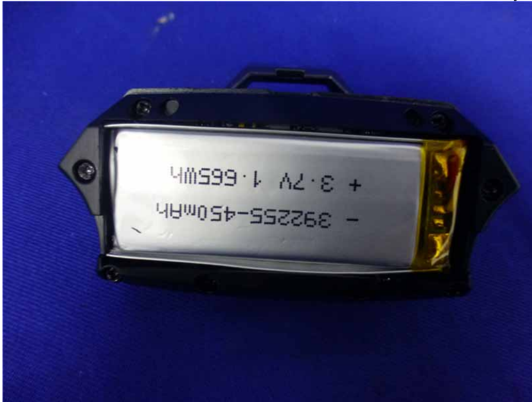
Figure 15 Battery of the EUT
