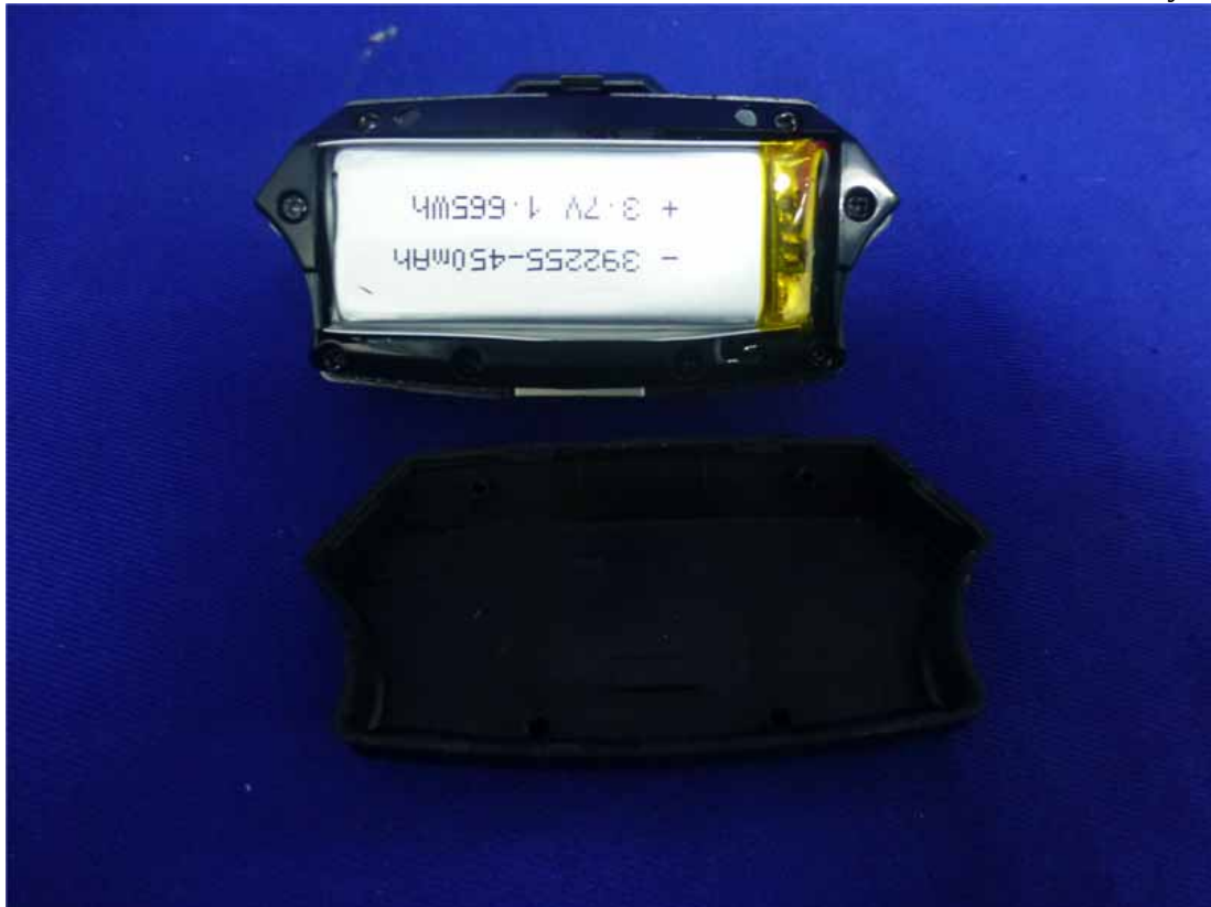
Figure 14 Battery of the EUT
