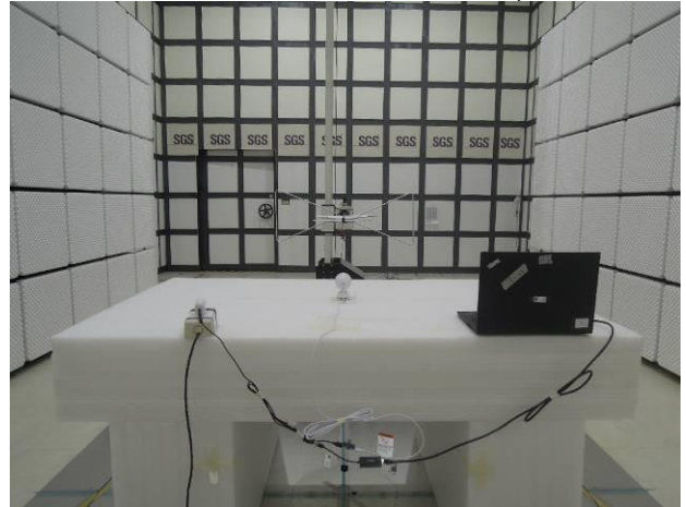
FCC 15 247 WLAN Radiated_Setup
