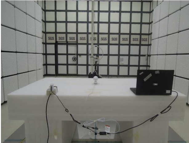
FCC 15 247 WLAN Radiated_Setup
