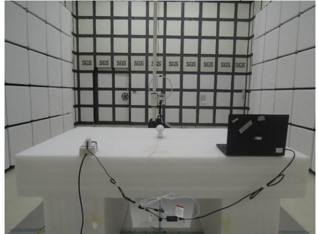
FCC 15 407 WLAN Radiated_Setup
