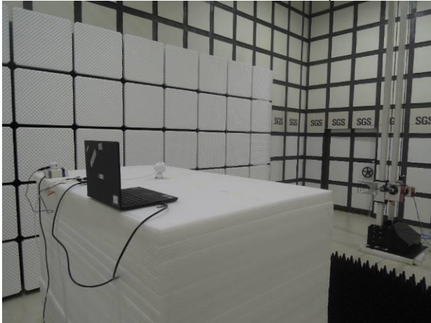
FCC 15 247 WLAN Radiated_Setup
