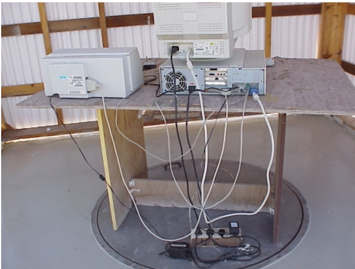
Photo #2. Radiated emission setup
