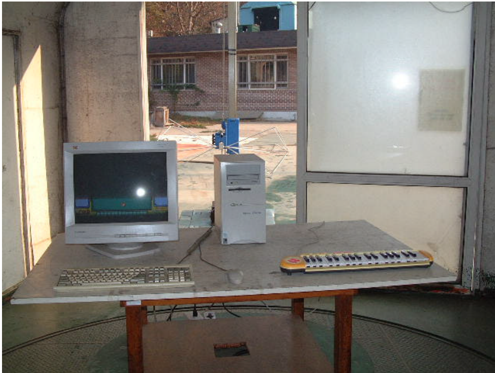
RADIATED EMISSION SETUP PHOTOGRAPH - FRONT VIEW ( 30 - 300 MHz )
