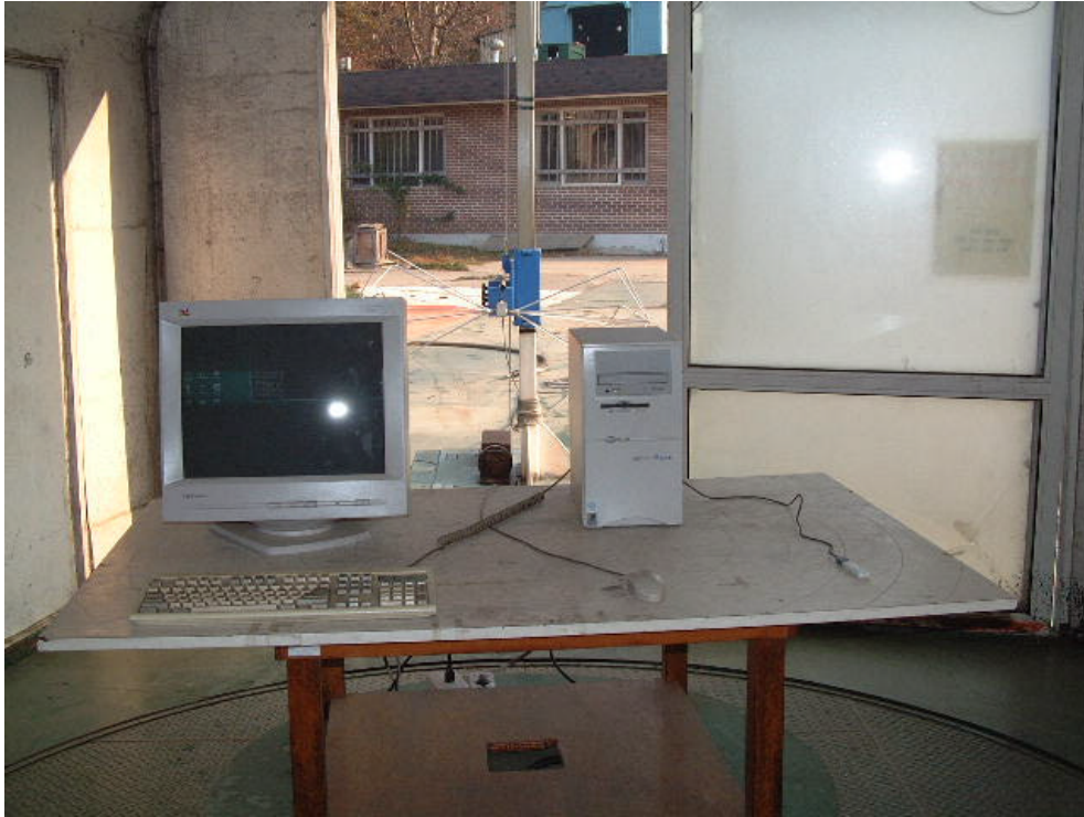
RADIATED EMISSION SETUP PHOTOGRAPH - FRONT VIEW ( 30 - 300 MHz )
