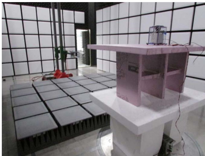
Figure 2: Radiated Spurious Emissions – Rear View – Above 1GHz
