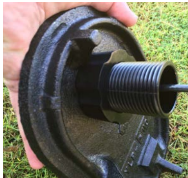
Figure 30 – Antenna Installation Complete
