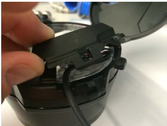
Figure 9 – Covering the Terminal Screws
