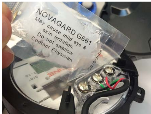
Figure 8 – Application of the Sealant
