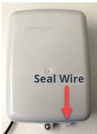
Figure 24 – Installing the Seal Wire
