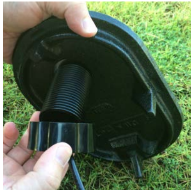
Figure 29 – Locking the Nut on the Antenna
