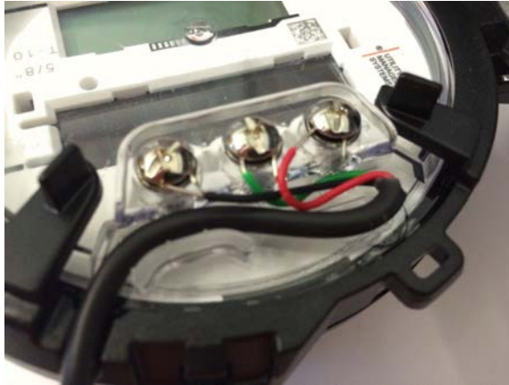
Figure 7 – Cable Threaded Around Strain Relief Posts
