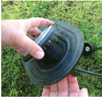
Figure 13 – Inserting the Antenna into the Pit Lid
