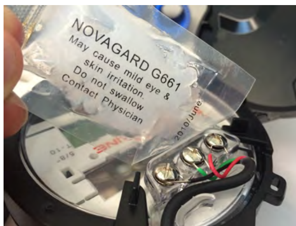
Figure 8 – Application of the Sealant
