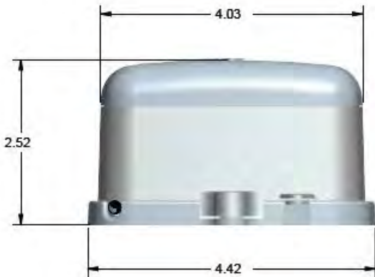
Figure 3 – L900 MIU Pit Dimensions - Side
