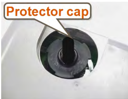
Figure 17 – Black Thread Guard from Male F-Connector
