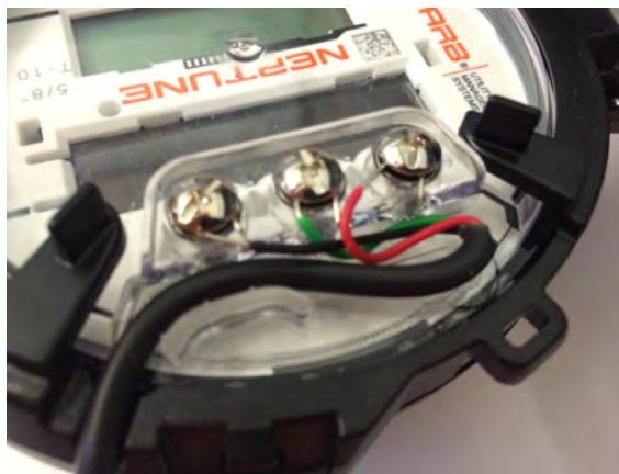
Figure 7 – Cable Threaded Around Strain Relief Posts
