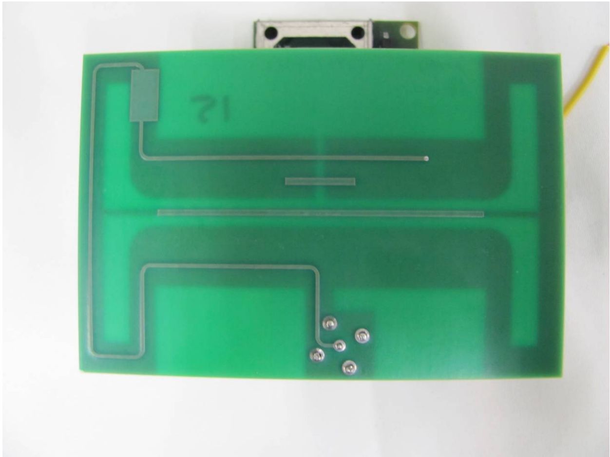
Figure 7. Wall Antenna, Front
