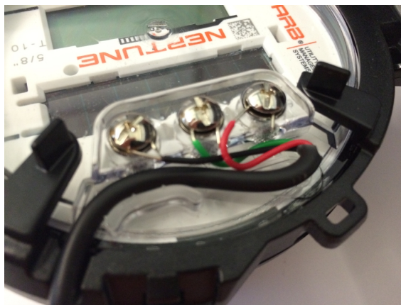
Figure 10 – Cable Threaded Around Strain Relief Posts
