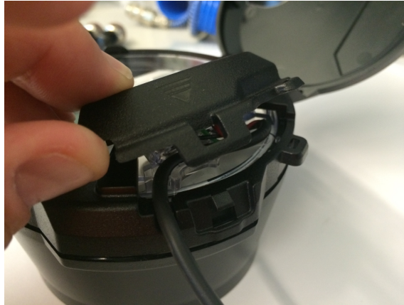
Figure 12 – Covering the Terminal Screws
