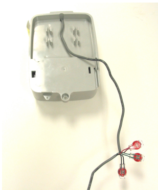
Figure 16 – Gel Cap Connections
