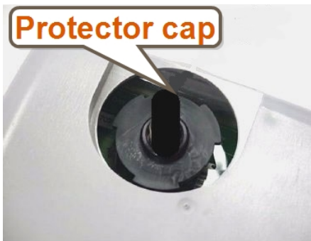
Figure 30 – Black Thread Guard from Male F-Connector
