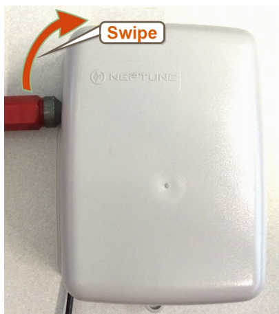
Figure 45 – Magnet Swipe the L900 MIU
