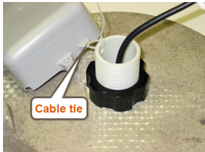
Figure 44 – L900 MIU Attached to Antenna
