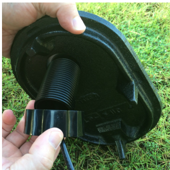
Figure 27 – Locking Nut on Antenna
