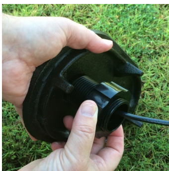
Figure 28 – Securing the Locking Nut
