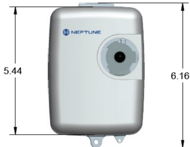
Figure 3 – L900 MIU - Pit Dimensions - Front
