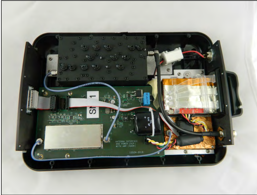
Figure 1: Internal Photo – MRX920v3 Assembly – Top Cover Removed
