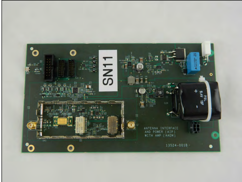
Figure 14: Internal Photo – AIP PCBA (Top) without Shield
