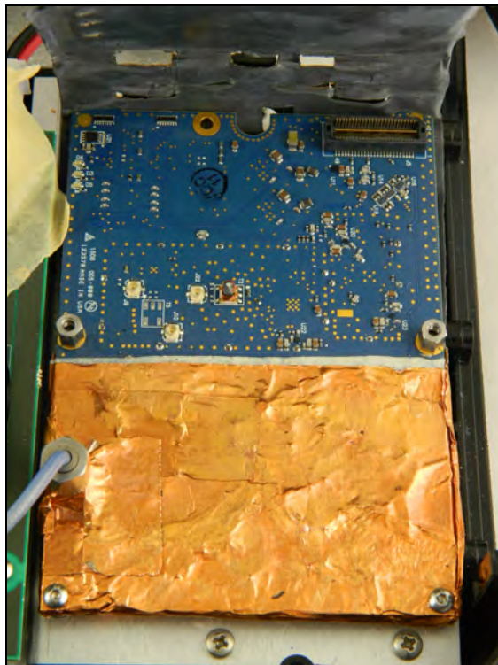
Figure 9: Internal Photo – RF PCBA with Foil Shield Backed with Insulator
