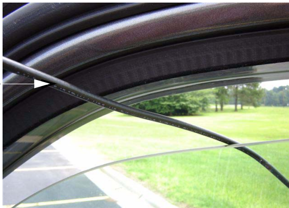
Figure 3.9 Antenna Cable Through Window
