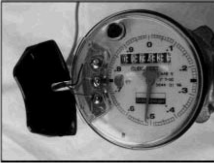
Figure 2.7 Covering the Terminal Screws
