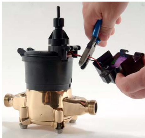
Figure 12 Cutting the Battery Wires
