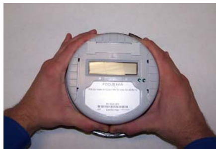
Figure 7 – Removal of Electronics Housing
