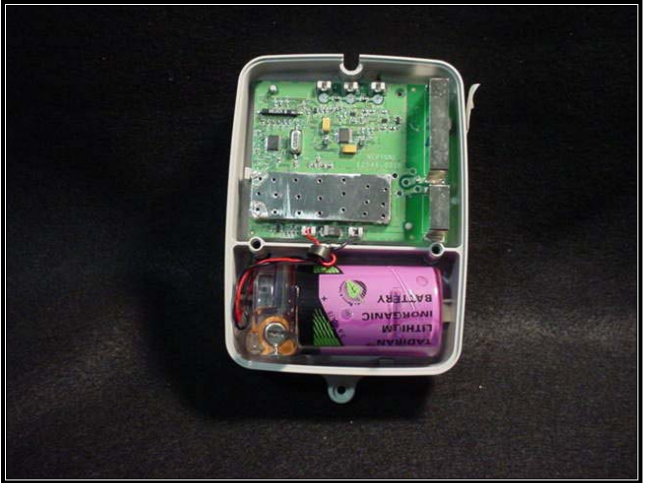
Figure C5: Wall Unit – With Cover Removed
