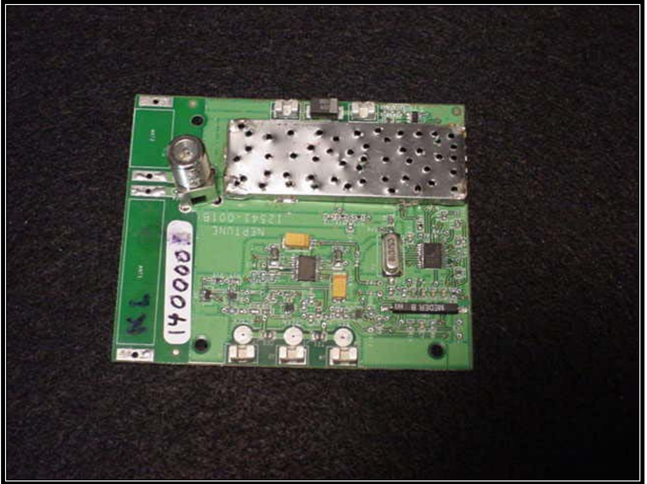
Figure C2: Pit Unit Board – Top View with Shield
