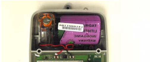
Figure 14 Returning Spliced Battery to Main Housing
