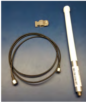
Figure 10 – Items for Cellular Antenna
