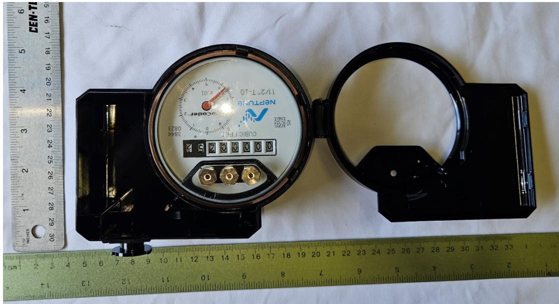
Figure 1. EUT, Cover Removed and Empty
