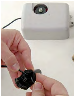
Figure 11 – Gray Wires in Slot
