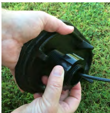
Figure 17 – Securing the Locking Nut
