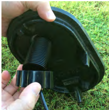
Figure 16 – Locking the Nut on the Antenna
