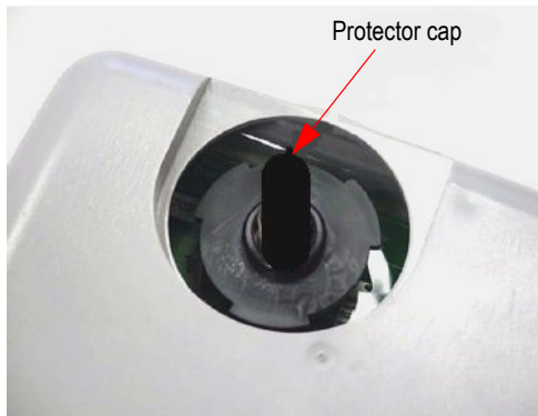
Figure 30 Black Thread Guard from Male F-Connector
