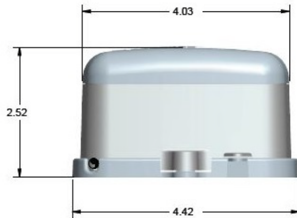
Figure 4 Pit MIU Dimensions - Diagram 2
