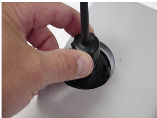
Figure 34 Black Cone-Shaped Gasket and Connector
