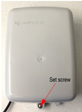
Figure 20 Securing Mounting Adapter
