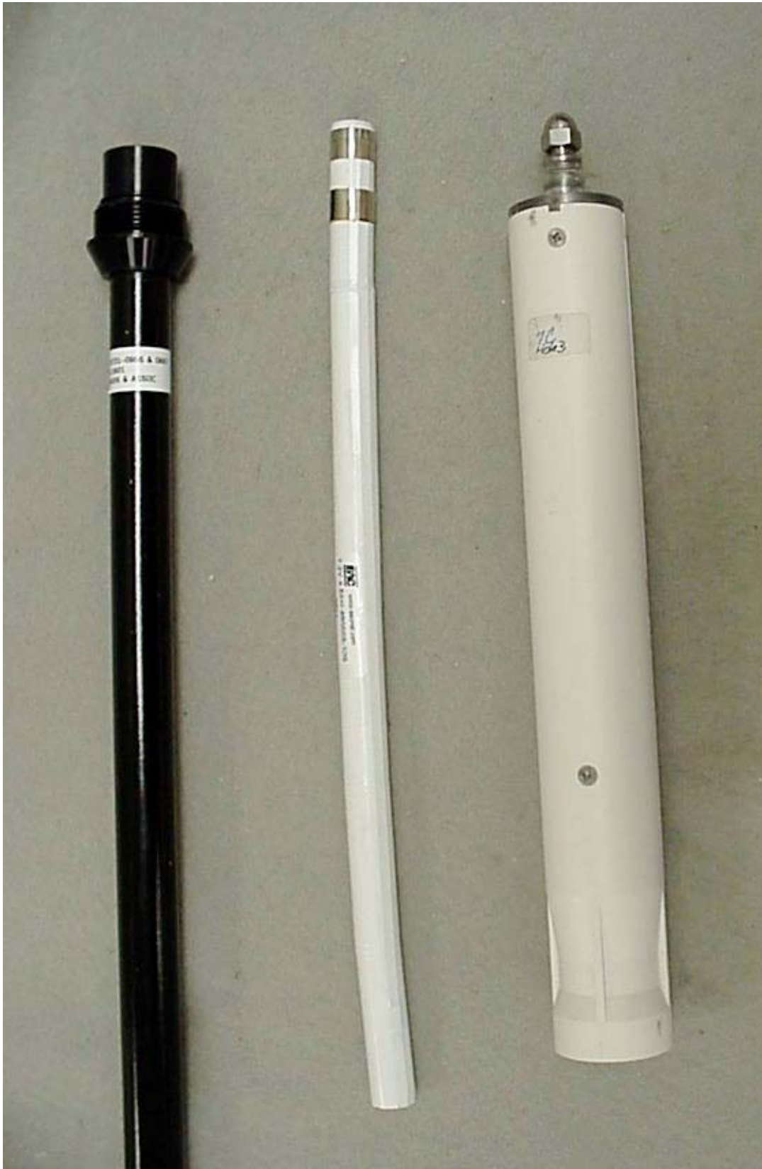
Photo 2. Exploded View of Flag Pole, Battery, & EUT
