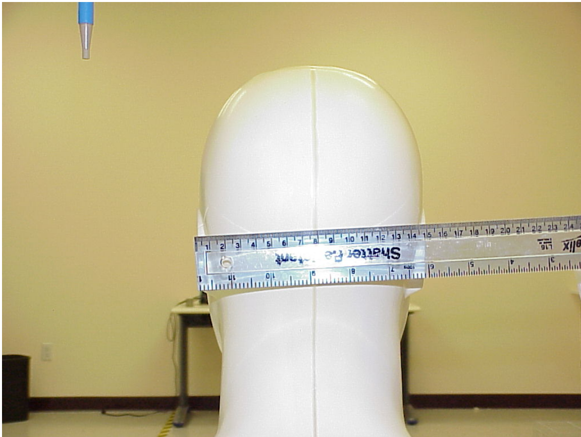
Photo 8. Photo to demonstrate 15 cm Z-axis head phantom
