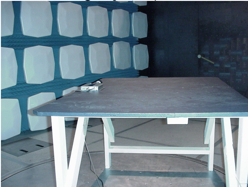
Article 33- Picture: EUT @ 90 Degrees; Set-up in 3-meter chamber
