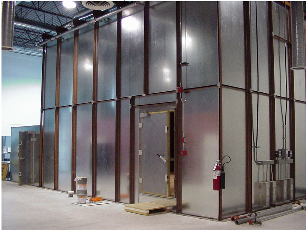
Article 10 - 3m Semi-anechoic chamber, Exterior view
