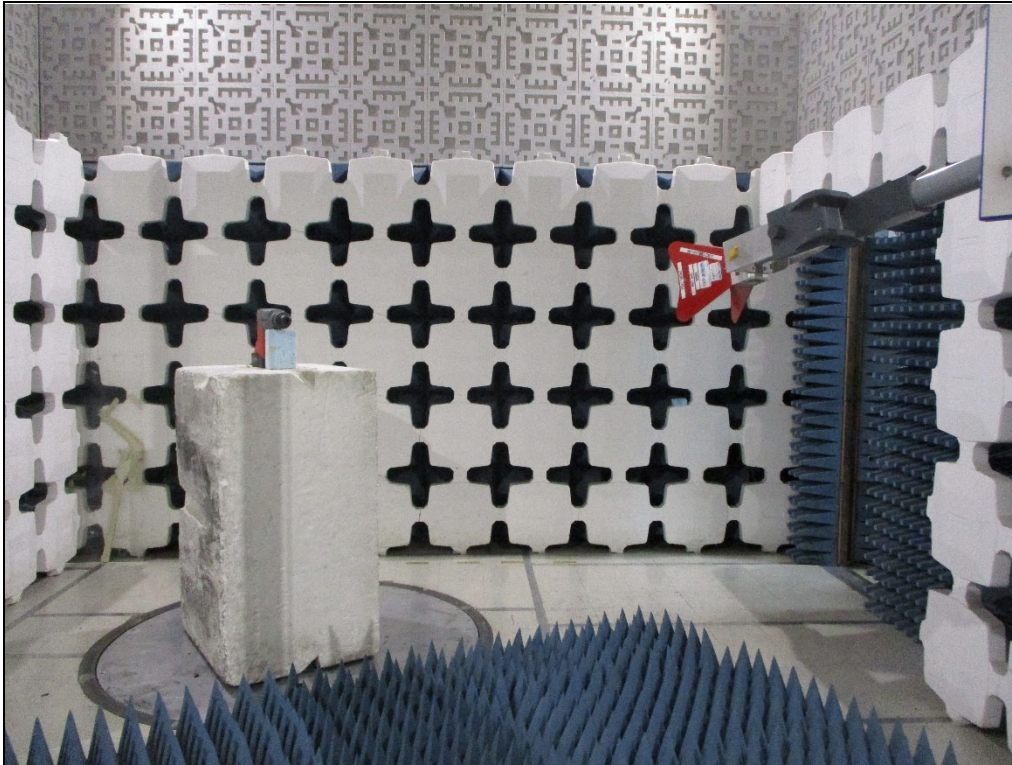
Test Setup for Spurious Radiated Emissions, Above 1 – 18GHz – Antenna Polarization Horizontal
