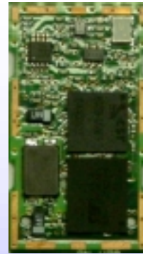
BTM2010-1(+20dBm) 35mm x 17mm x 2.6mm
