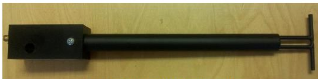
Figure 1 – MVG COMOSAR Validation Dipole
