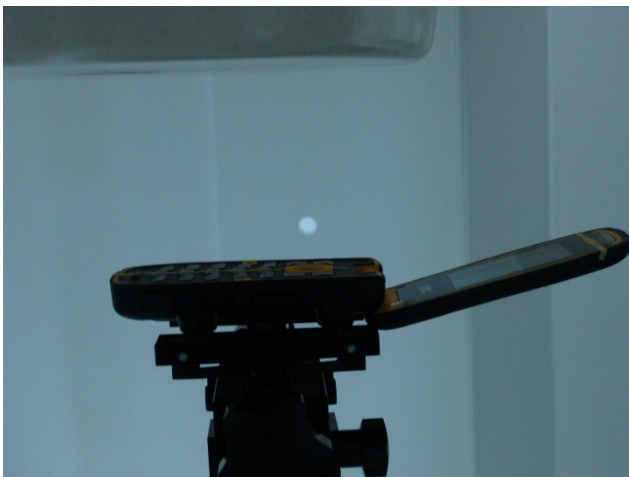
Right Tilted position - Separation distance 7.8cm between mouth and antenna
