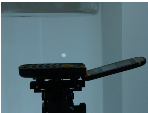
Left Tilted position - Separation distance 8.0cm between mouth and antenna
