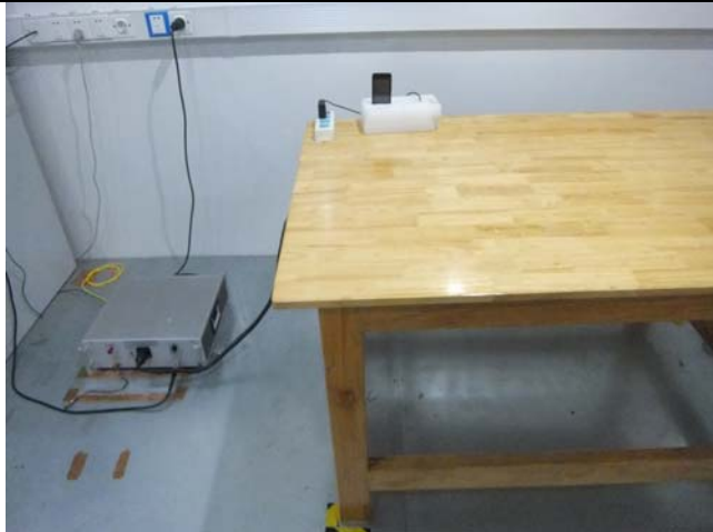
Conducted Emissions Test Setup Front View
