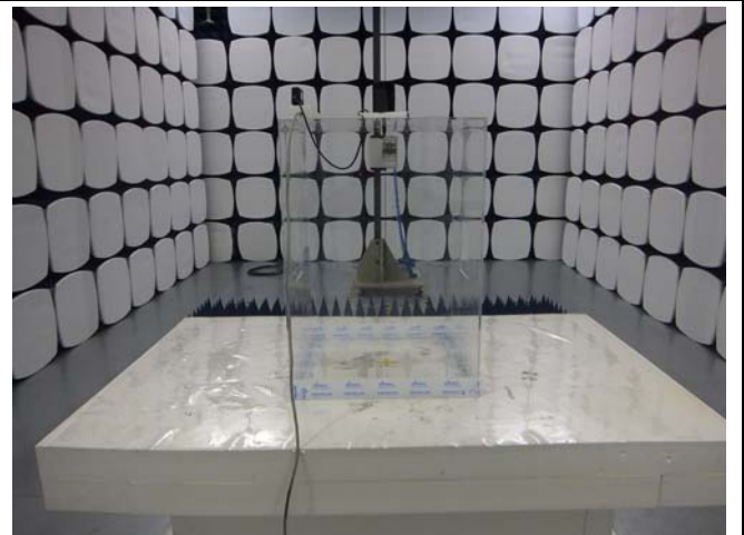
Radiated Spurious Emissions Test Setup Above 1GHz
