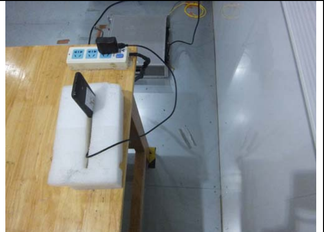
Conducted Emissions Test Setup Side View
