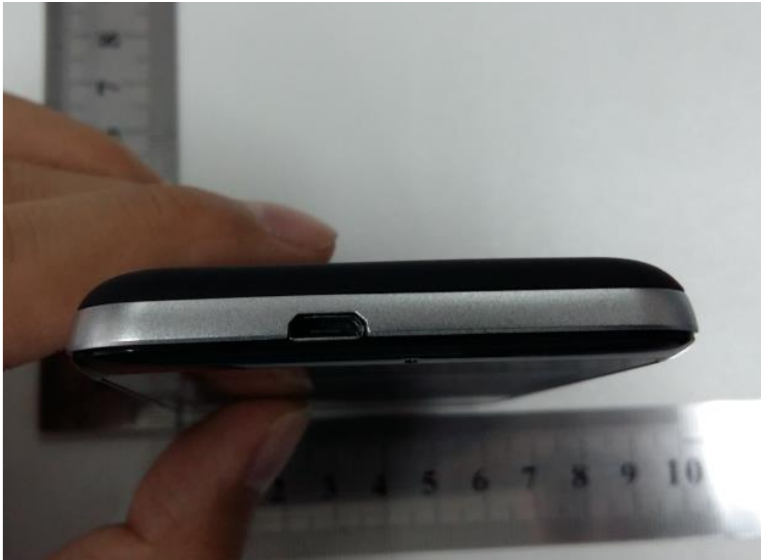
Figure 7 U307TG, MXG308 bottom Micro USB charger connector
