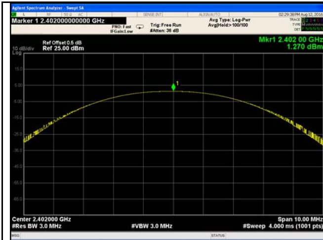
8DPSK Output power - Low CH 2402
