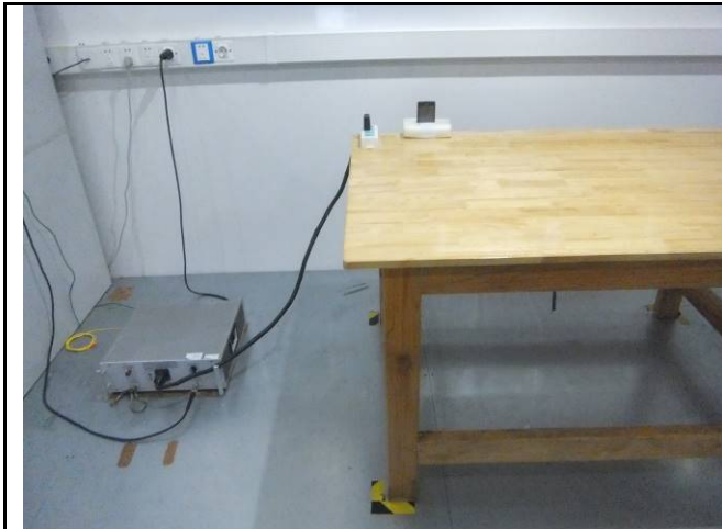
Conducted Emissions Test Setup Front View
