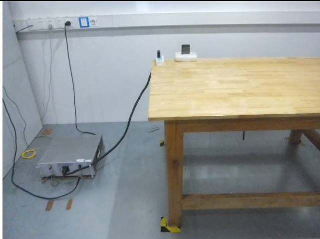
Conducted Emissions Test Setup Front View
