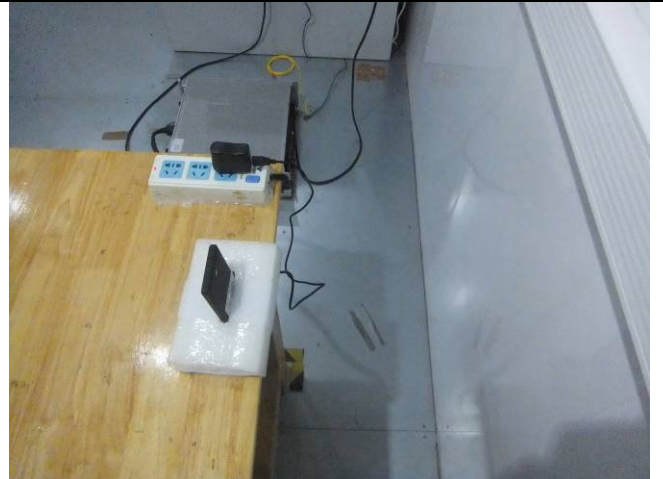
Conducted Emissions Test Setup Side View
