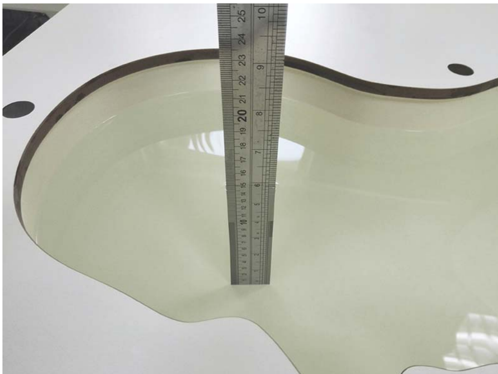
Liquid depth in the head Phantom (1900 MHz, 15.1cm depth)
