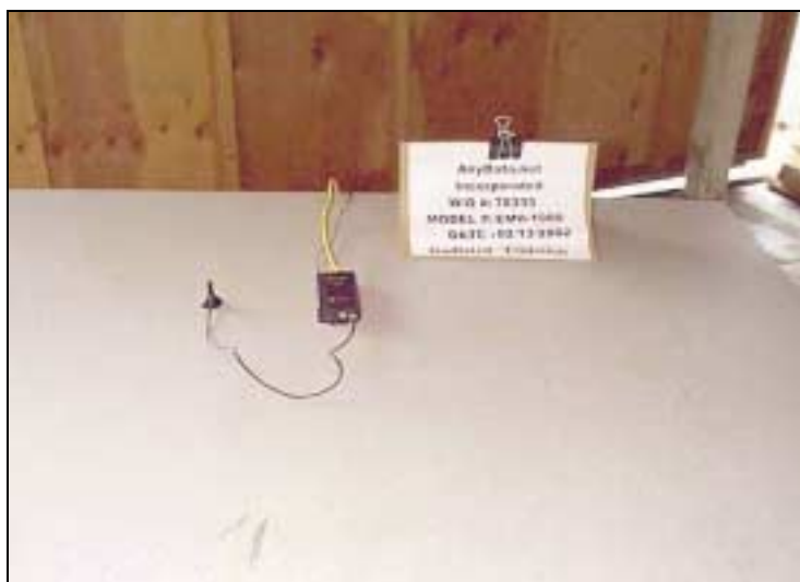
OATS Test Setup – Front View
