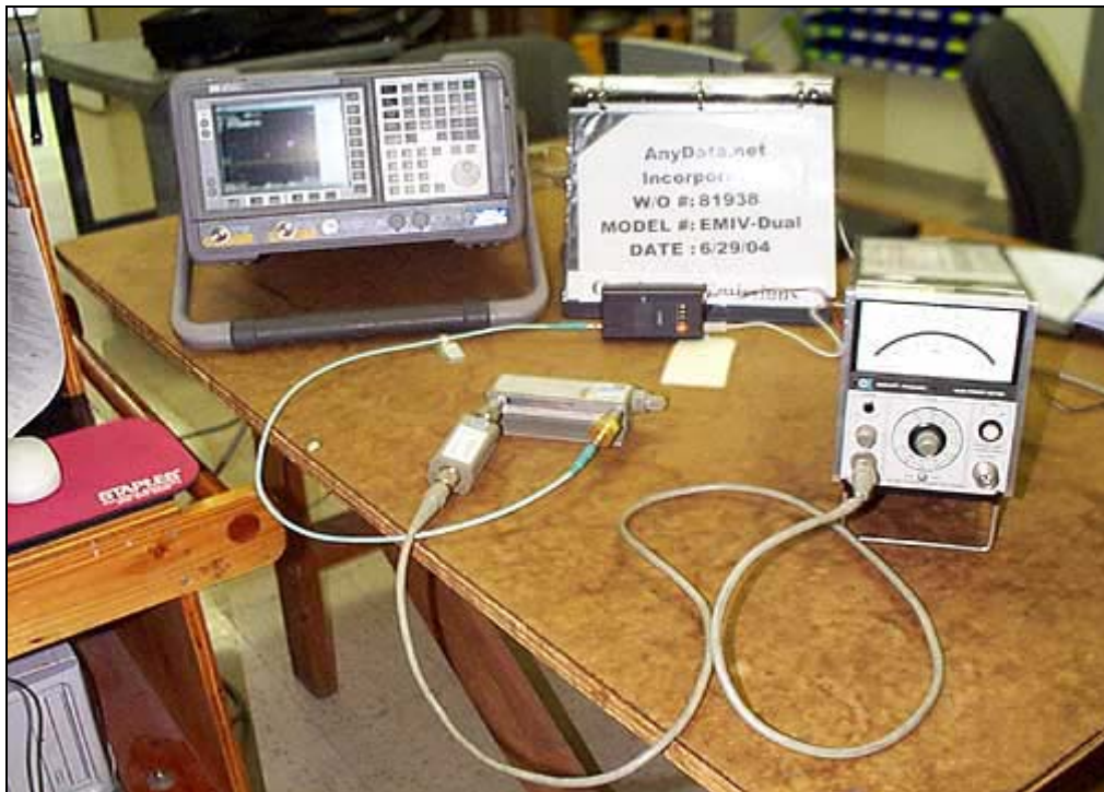
PHOTOGRAPH SHOWING DIRECT CONNECT TEST SETUP
