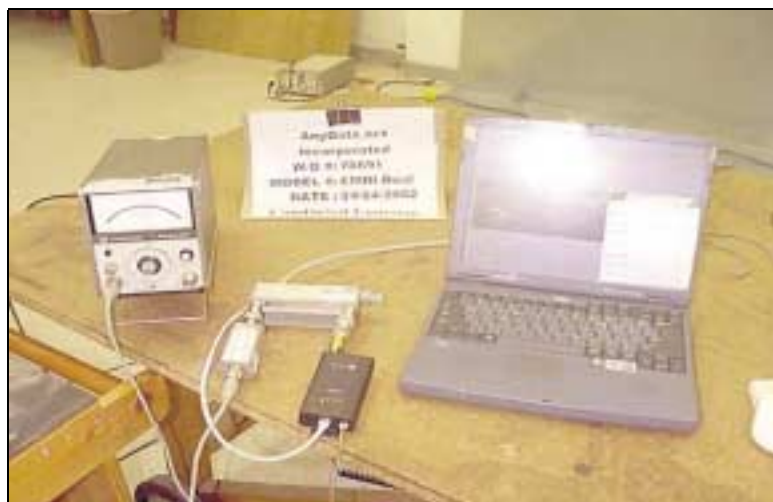
Carrier Output Power Test Setup
