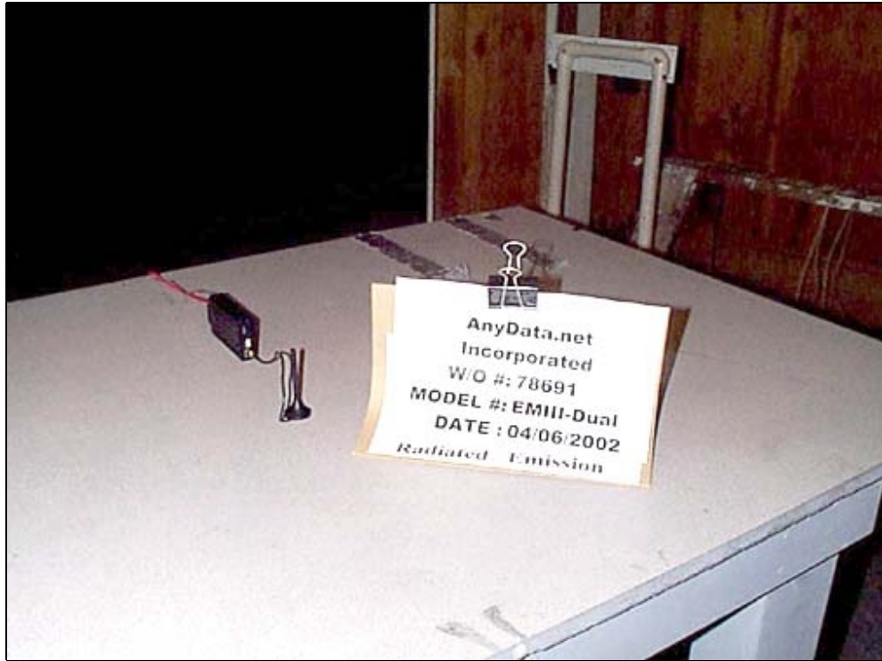
OATS Test Setup - Side View
