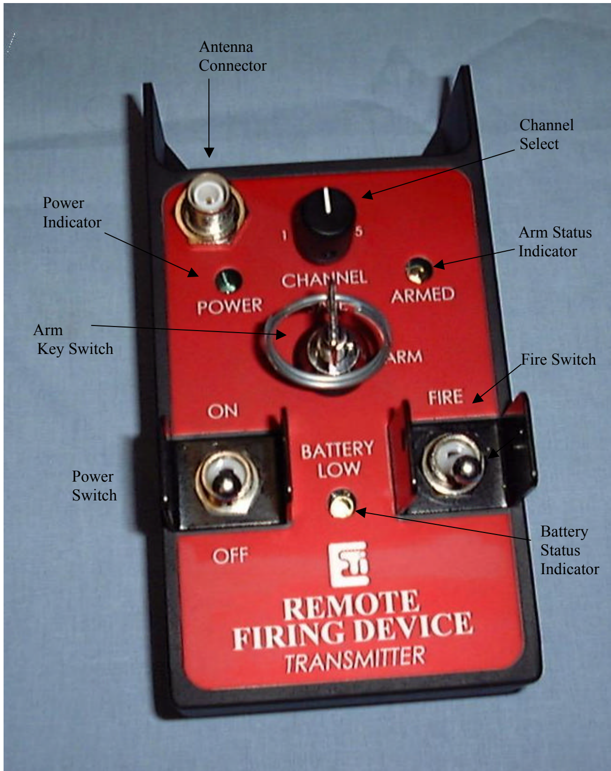
Figure 6. RFD transmitter unit controls and indicators.
