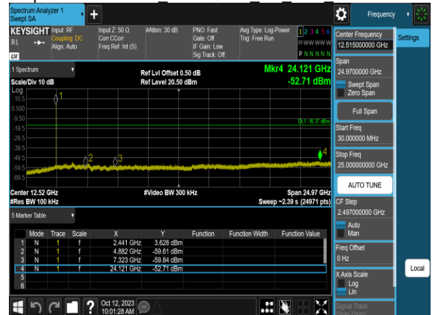
Spurious Emission \pi/4 DQPSK 2M DH5 2480MHz
