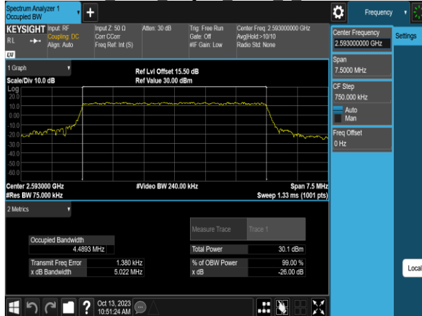
Band41 5MHz 16QAM RB25 0 CH41565
