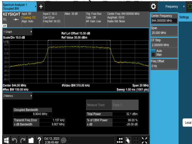
Band26 10MHz 16QAM RB50 0 CH26990
