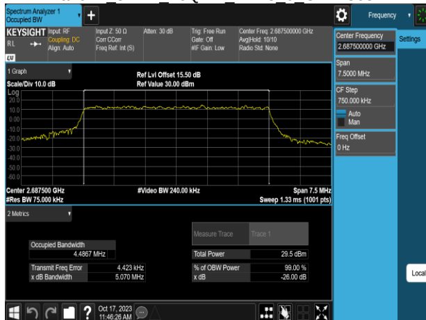
Band41 5MHz 64QAM RB25 0 CH39675
