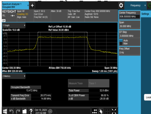
Band26 15MHz QPSK RB75 0 CH26965
