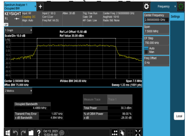
Band41 5MHz 64QAM RB25 0 CH41565
