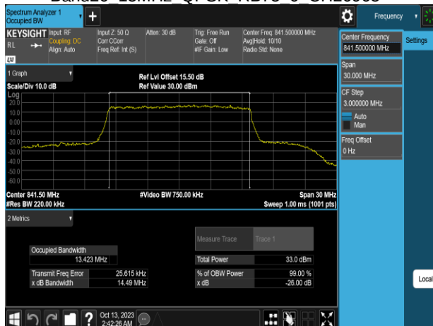
Band26 15MHz QPSK RB75 0 CH26965
