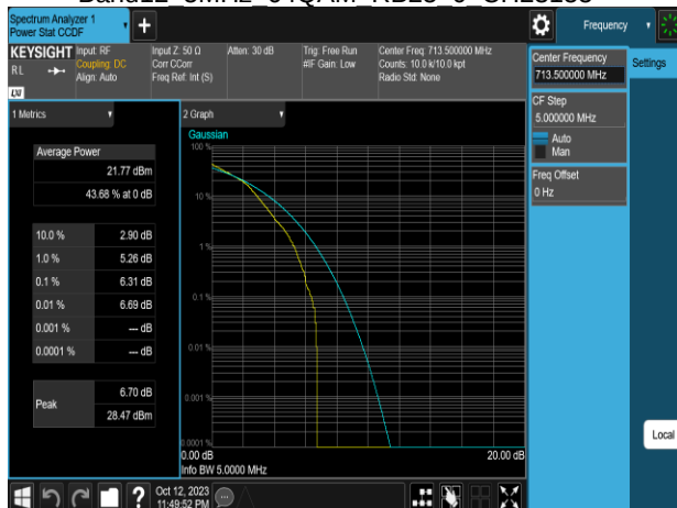
Band12 5MHz 64QAM RB25 0 CH23155
