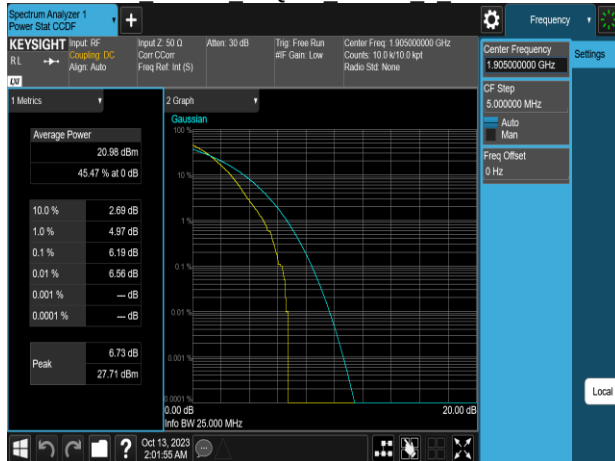
Band26 1.4MHz 64QAM RB6 0 CH26797
