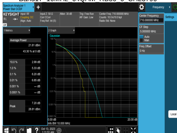
Band17 10MHz 64QAM RB50 0 CH23800
