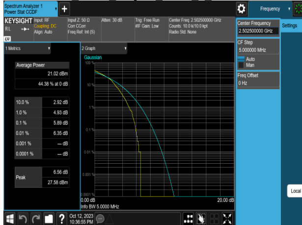
Band7 5MHz 64QAM RB25 0 CH21100
