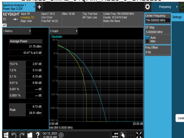
Band13 5MHz 64QAM RB25 0 CH23255
