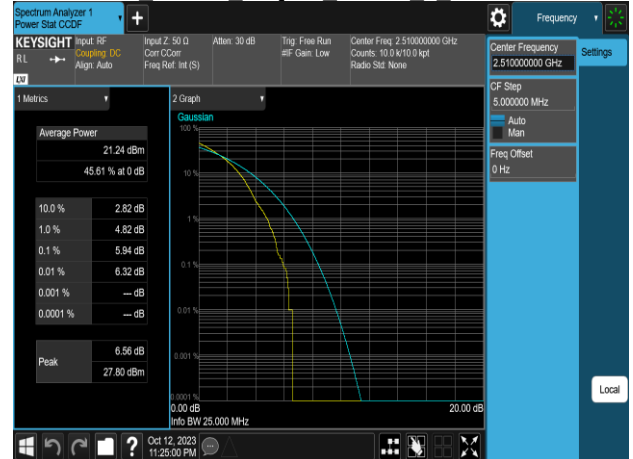
Band7 20MHz 64QAM RB100 0 CH21100
