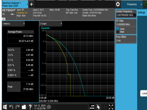
Band7 15MHz 64QAM RB75 0 CH21100
