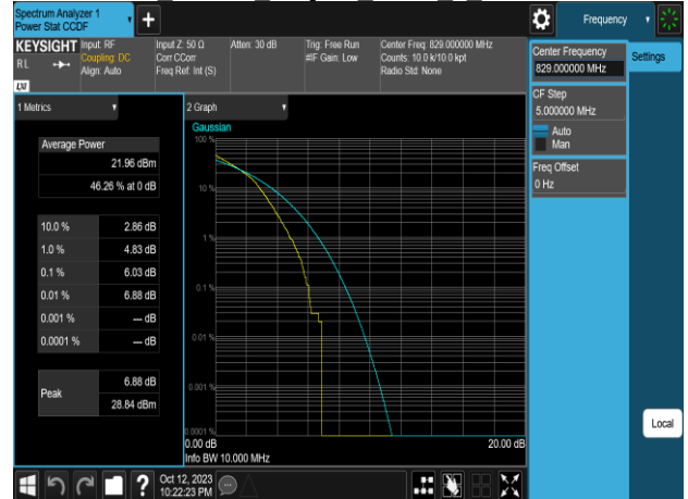
Band5 10MHz 64QAM RB50 0 CH20525
