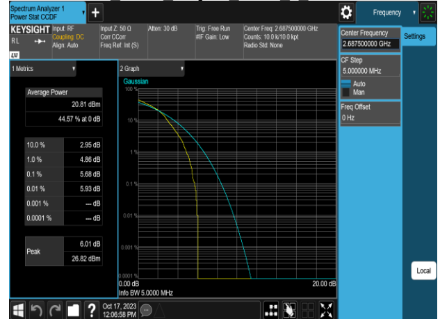
Band41 10MHz 64QAM RB50 0 CH39700
