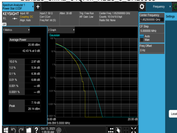
Band25 5MHz 64QAM RB25 0 CH26065
