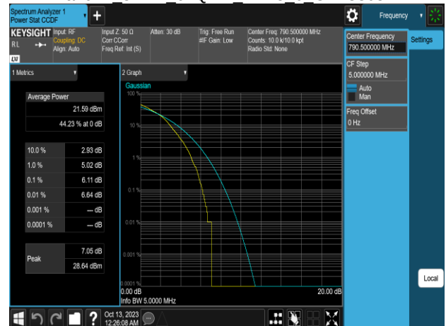
Band14 5MHz 64QAM RB25 0 CH23330
