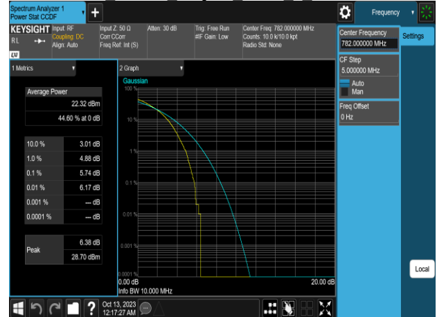
Band14 5MHz 64QAM RB25 0 CH23305
