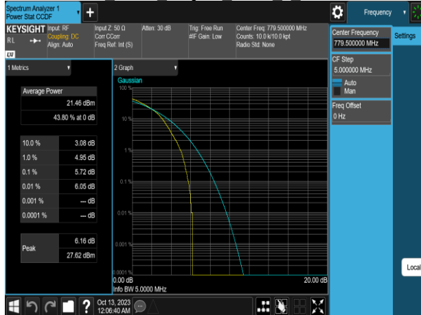
Band13 5MHz 64QAM RB25 0 CH23230
