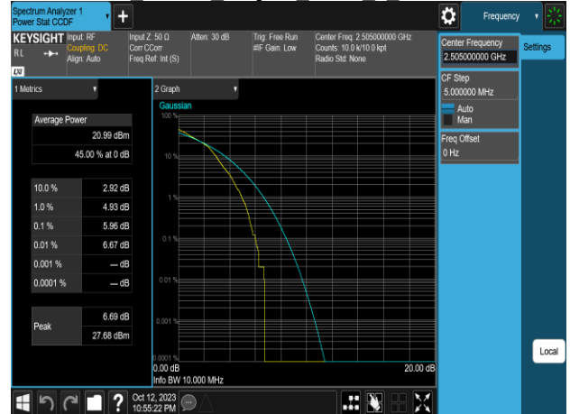
Band7 10MHz 64QAM RB50 0 CH21100
